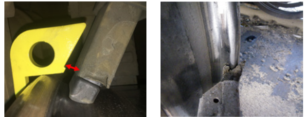
Figure 5. Examples of misaligned on-board flange lubrication.
