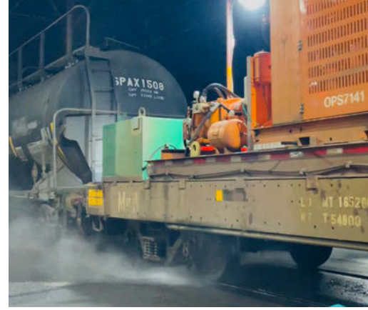
One of SEPTA's three trains that clean the rails to combat slip-slide.
