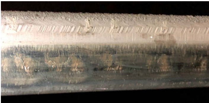
A series of squats appeared on the surface of un-ground rail.
