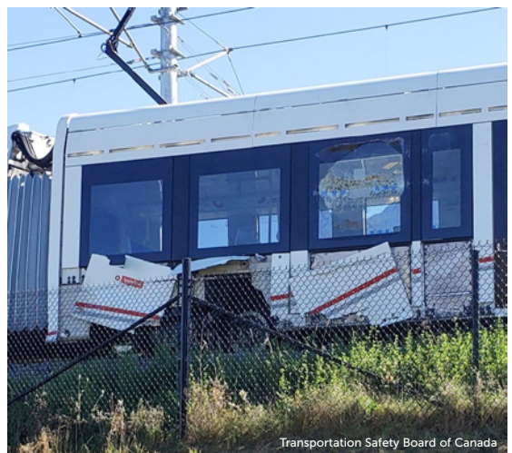
AN IMAGE showing damage to an O-Train following a September 2021 derailment that TSB determined to be caused by 12 bolts that failed because they were not adequately torqued when installed during refurbishment.
