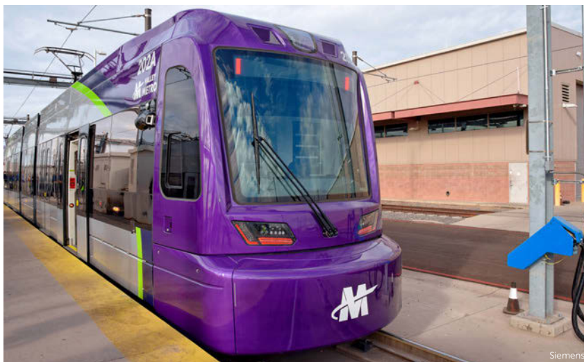
LRVS IN Phoenix feature a new front-end bumper designed to minimize collision impact and vehicle damage while increasing operator and passenger safety.
