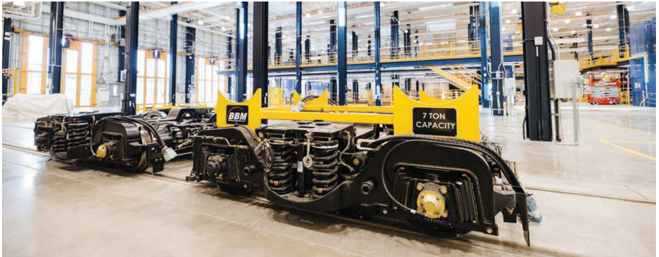
LIGHT-RAIL VEHICLE trucks await installation in the Sound Transit Operations and Maintenance Facility East.
